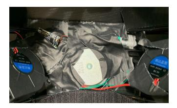
we've removed the chin rest on the mask here for easier access. Don't forget to put it back. We've also added some tape over the fan leads because those are common failure points.
