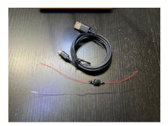
switch wire and the negative power wire to the 7" black lead. Protect the connections with heat shrink and set aside for final electronics assembly.
