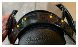
These are for attaching the speaker (middle holes) and the eye mount plate (outside holes)
