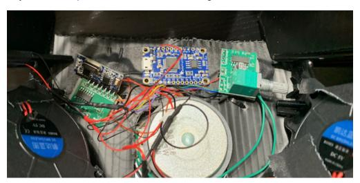
At this point, you may want to connect a battery and retest the system to make sure you haven't dislodged a wire. If all works well, secure the wires with tape. Note that there are lights on the sound board and remote receiver that you may wish to cover to avoid their glow lighting your face. You may wish to leave the USB jack on the soundboard accessible in order to change your sounds. Note that
