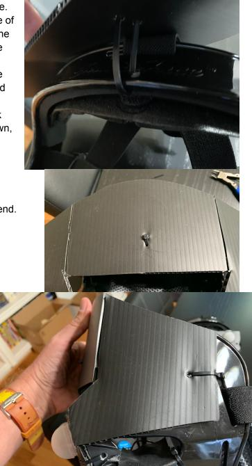
This is also a good time to "seal" the area around the fans with tape. This isn't critical *per se*, but it does help to make sure that the fans pull air through the mask's fabric cover instead of just blowing are around inside the mask. No need for perfection, just try to seal air gaps and don't stop the fan from rotating. Pics below.
